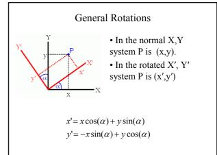
Rotation Matrices – 2D Rewriting as a matrix equation  $\begin{pmatrix} x' \\ y' \end{pmatrix} = \begin{pmatrix} \cos(\alpha) & \sin(\alpha) \\ -\sin(\alpha) & \cos(\alpha) \end{pmatrix} \begin{pmatrix} x \\ y \end{pmatrix} = R_{\alpha} \begin{pmatrix} x \\ y \end{pmatrix}$ The operation "rotate the coordinate system anti-clockwise by a", is identical to "rotate objects clockwise by a" The operation is implemented by multiplying
